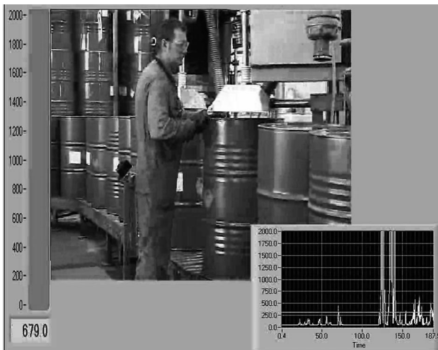
Fig. 2. Example of a PIMEX screen. The video picture window shows a person filling cans with acetone and carrying a monitoring instrument for solvents. The graph window shows how the operator's exposure to acetone has varied during the period. The gray bar to the left shows the current exposure level, which is very high.
